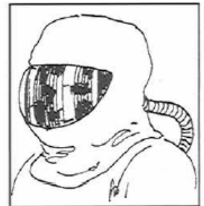
THIS TYPE SUPPLIES CLEAN AIR. Airline hood respirator (for very high dust levels).
