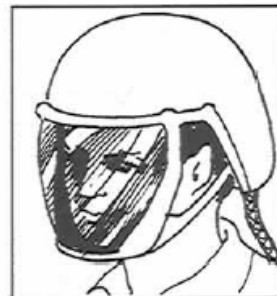
THIS TYPE FILTERS THE AIR. Battery powered respirator (for medium dust levels)
