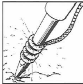
Water coil attachment to suppress dust on jackpicks and scabbling picks, and watersprays fitted to rockbreakers.
