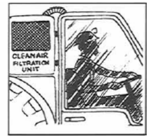
Cabs fitted with air-filtration (not ordinary air-conditioners - they do not trap very fine dust).
